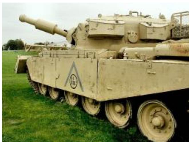
At the Land War Exhibition. A Centurian Mark 5 AVRE (Assault Vehicle Royal Engineers) featuring a bulldozer blade and a 165mm demolition cannon
